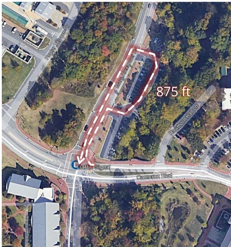
Figure 22. Map showing the U-turn at Lot 12 to enable the shuttle to navigate through the intersection at Cameron Boulevard and Mary Alexander Road without turning left at the traffic signal. (Image courtesy of NCDOT using Google Earth)
