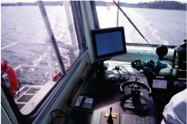
New vessel monitor and bridge controls
