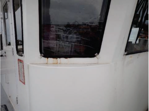
Typical condition around windows as vessels age
