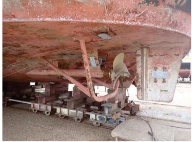
One of rudders for twin screw vessel
