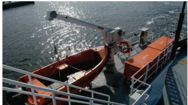
New rescue boat with now-standard quick release hook
