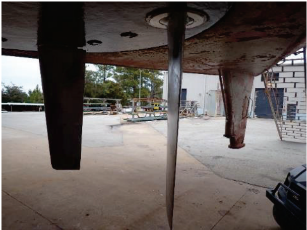
Voith unit with fin, but not rudder
