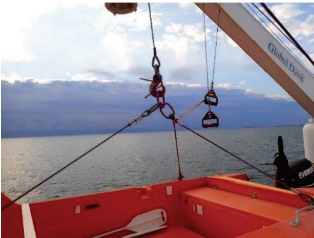
Older style non-quick release hook for rescue boat
