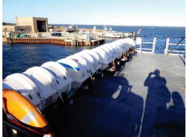
Standard configuration of life rafts on racks with hydrostatic releases
