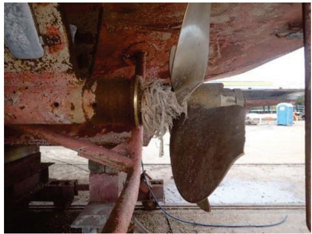
Screw of twin screw vessel with rope fouling
