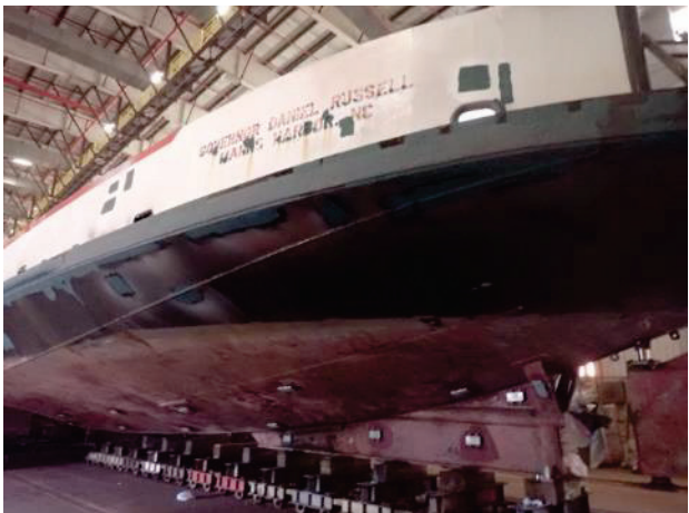
Hull being prepped with new zinc anodes visible
