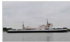
Sound Class , the largest ferries, are designed for the turbulent waters of the Pamlico Sound; these ferries can carry as many as 48 vehicles and 300 passengers.
