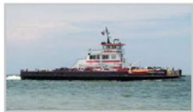
Hatteras Class , the smallest ferries, carry 24 vehicles and 149 passengers and are specifically designed to ply the shallow waters of eastern North Carolina.
